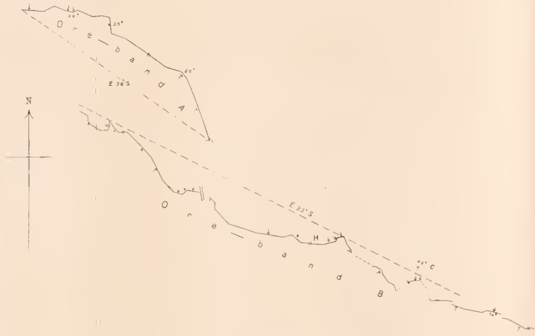
FIG. 2.—PLAN SHOWING THE EXTREMELY VARIABLE STRIKES AND DIPS OF THE TWO ORE-BANDS AT MANDRI, NAGPUR DISTRICT.
